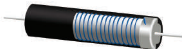
Figure 2: The fundamental construction of a wirewound resistor has changed little over time.
